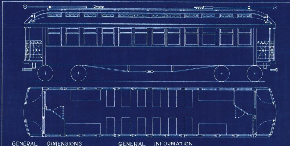
LENGTH OVERALL 46'-02" LENGTH OVER BODY 38-10" HEIGHT RAIL TO TOP OF ROOF 12'- 62 HEIGHT RAIL TO BOTTOM SILLS 2'- 10" HEIGHT FLOOR TO CEILING 8'-93" EXTREME WIDTH WIDTH OVER SIDE SHEATHING 8'- 74 WIDTH OVER UPPER DECK 5'-6" WIDTH BETWEEN CROSS SEATS 172" WIDTH BETWEEN LONG. SEATS 3'-104" SEATING CAPACITY END DOOR OPENING
