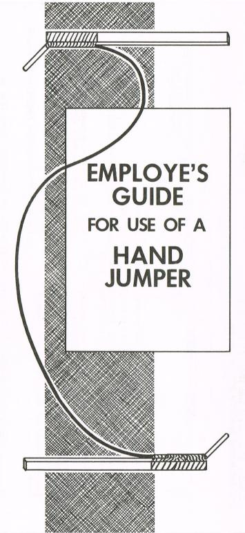
Whenever work involves making or breaking electrical circuits of high amperage, there is danger of an arc or flash. A Hand Jumper (stinger) improperly used can cause such an arc or flash. The purpose of this folder is to explain the procedures for using a Hand Jumper.
