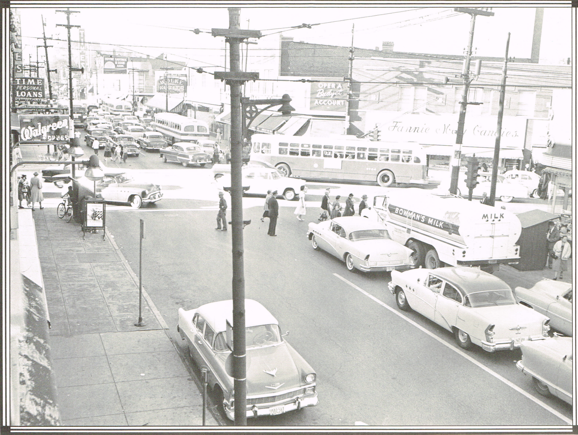
The Marmon-Herrington trolley bus, shown westbound on Lawrence at Milwaukee Avenue in 1956, seated 49 passengers, and was part of an order for 349 delivered in 1951-52. Propane buses provided a smooth ride on Milwaukee, where streetcars had operated only four years earlier.
