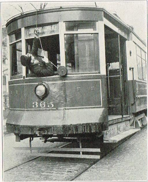
When the trolley is adjusted from this position, the conductor is in no danger of being injured.
