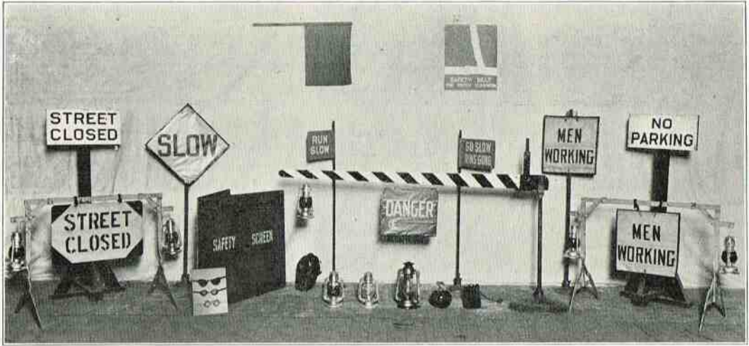
Types of Protective Warning Signs and Signs Used by the Track Department.
