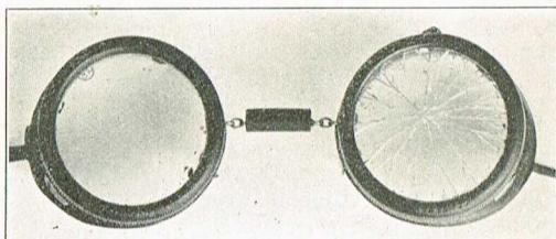
Following are five cases of men working with their goggles on when flying pieces of concrete shattered the safety lens, but causing no injury to the eye:
