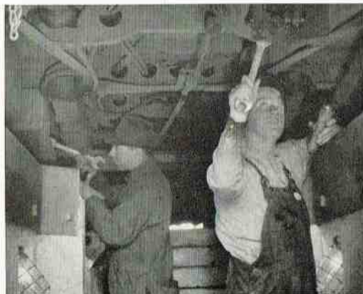
Down in the pit, Jack Jobaris (left) and Johnny Cahill adjust the bus's brakes.
