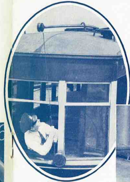
Conductor Ben Zentmeyer, Elston, shows how a trolley pole sometimes catches under the point, rather than in the hook.
