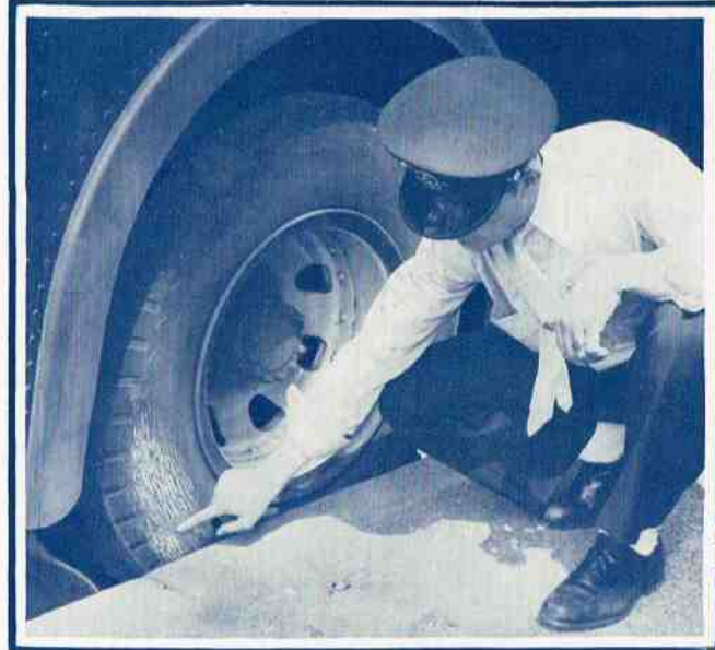
Bus Operator Charley Brisolara, Lawndale, examines a tire which has been badly scraped against the curb.
