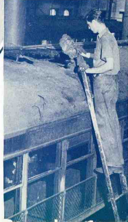
Conductor Ben Zentmeyer, Elston, shows how a trolley pole sometimes catches under the point, rather than in the hook.
