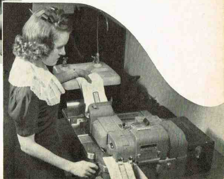
Helen operates the sealing and meter-printing machine which rapidly seals all envelopes and prints the proper postage on them.
