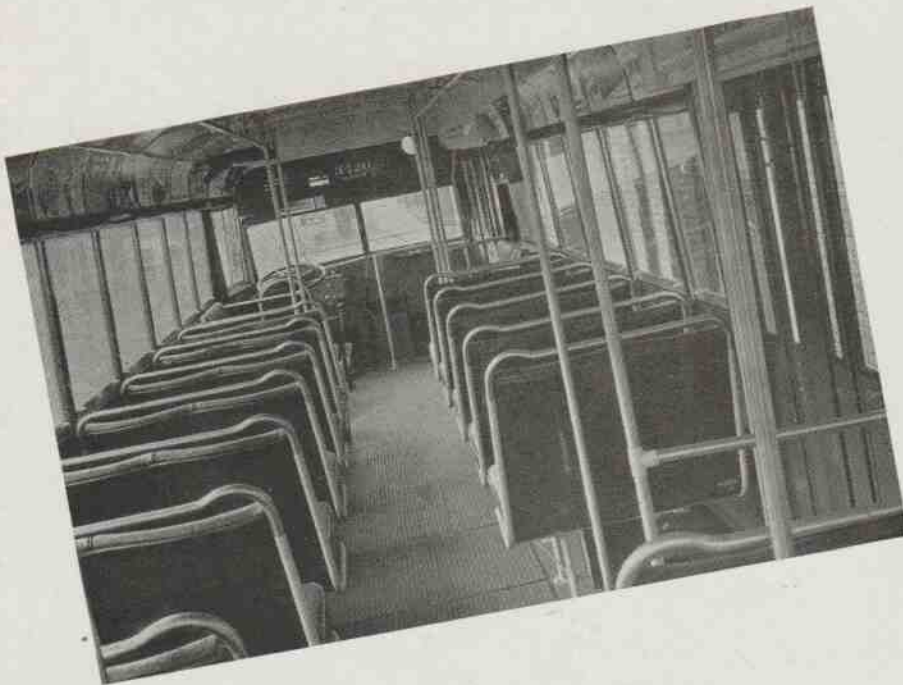
Upholstered in green leather, the White bus seats 44 passengers—more than the older streetcars. The eduction ventilating system assures comfortable air circulation—the motion of the bus taking out the air through ceiling vents.
