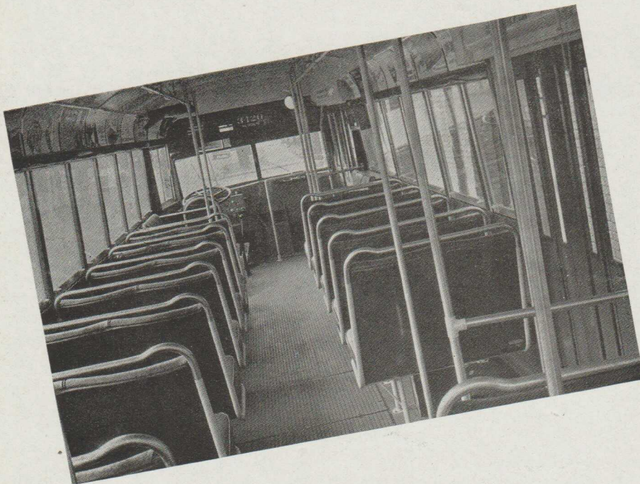
Upholstered in green leather, the White bus seats 44 passengers—more than the older streetcars. The education ventilating system assures comfortable air circulation—the motion of the bus taking out the air through ceiling vents.
