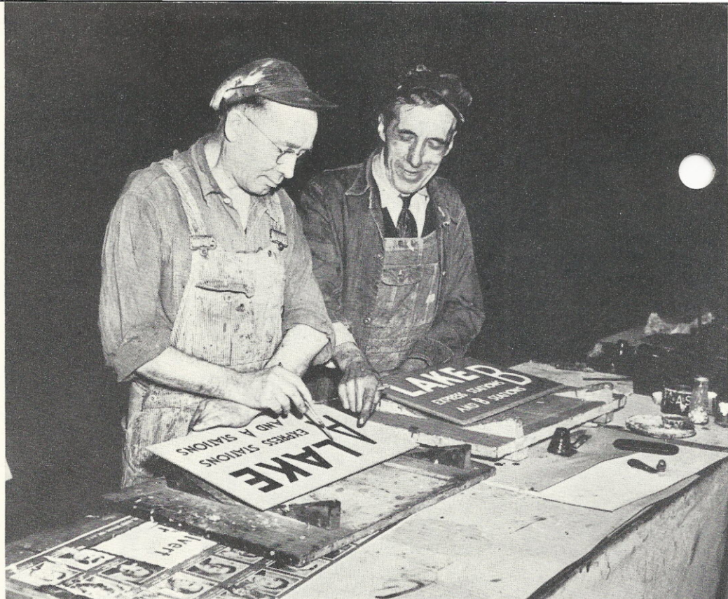
HEAD-END SIGNS for trains in the new Lake street "L" express service being made at the Skokie shops. Tony Janca (left) and Kolman Mager , both veteran "L" employes, add the finishing touches to the lettering. The signs were then varnished, frames added and metal reinforcements put on the corners.
