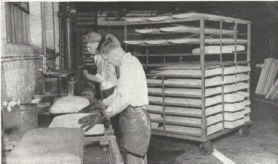
WHILE AN "L" car is moving through its stages of rehabilitation, the seats are also being renovated. Frank Thinner (front) and Bob Du Bois scrub and rinse the seats until they are gleaming.
