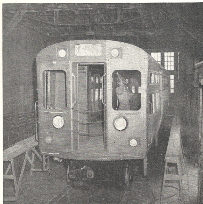
8. In the paint shop, both the interior and exterior surfaces of the shell are smoothed with a putty-like substance and sand-papered. It is then painted in CTA colors. In the finish shop the seats, lighting fixtures, door hardware, etc., are installed.
