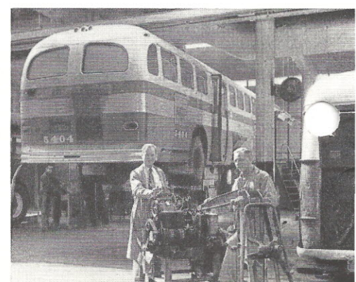
BUS MAJOR INSPECTIONS or overhauls are among the several functions of the pit and hoist area at West Shops. In this picture, Stanley J. Eisen (left), and Mitchell F. Kitzman , foremen, are checking a Ford engine assembly before installation in bus. →
