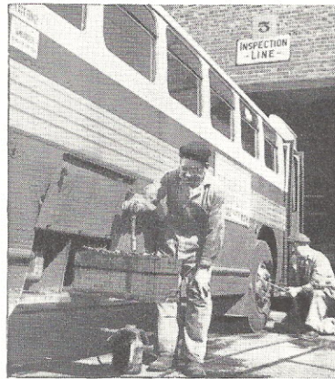
AS PART of a 2,000 mile inspection, Antonio DeBlasi (left), battery inspector, takes a hydrometer reading, and Patrick O'Malley tests tires at North Park.
