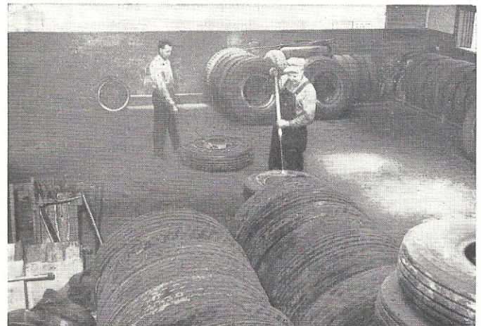
TIRES for approximately 800 trolley and gas buses are serviced in the tire repair room at North motor garage. Tire Repairman John Wolf , left, puts low-pressure air in a remounted tire as John Sullivan , tire repairman, removes a tire.
