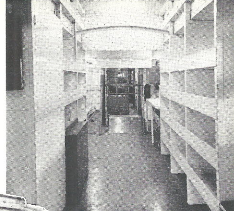
INTERIOR VIEW of new line car showing shelves and bins for material and tool storage.
