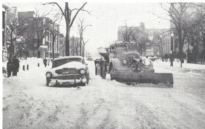
A CTA service truck, equipped with a snow-plow attachment, clears the way along Sheridan road between Irving Park and Montrose avenues. Again a parked car at the curb narrows the street area in which the plow can work.
