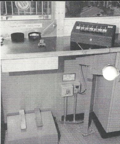
CLOSEUP VIEW of the top panel of the new Visi-Fare turnstile. When agent presses control key in booth, the corresponding fare is registered and compartment on top of the turnstile lights up to show what the customer paid.
