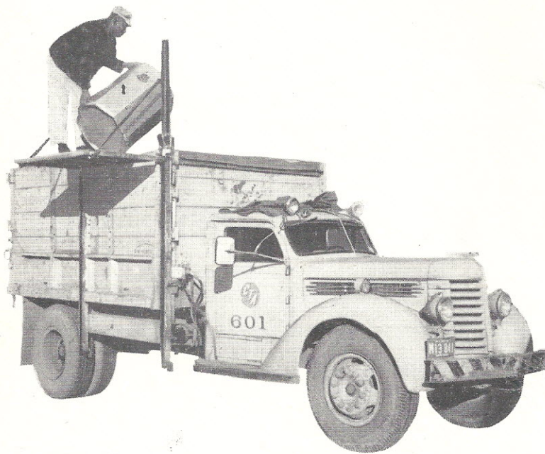
IN ORDER to increase the load capacity of the older equipment, the bodies of two five-ton dump trucks were converted by adding sideboards fitted above the metal section of the truck bed. Richard Farley , chauffeur, demonstrates how containers are emptied by use of a side-loader lift.
