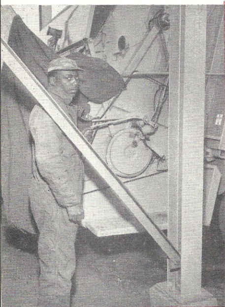
IN ORDER to increase the load capacity of the older equipment, the bodies of two five-ton dump trucks were converted by adding sideboards fitted above the metal section of the truck bed. Richard Farley , chauffeur, demonstrates how containers are emptied by use of a side-loader lift.
