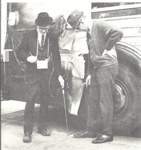
W. T. UNWIN (left) fire prevention and industrial safety coordinator, uses a combustible gas and vapor detector to check drains and low areas in the Paint Shop for combustible concentrations or vapors. Looking on is Ted Pietrus, paint shop foreman.
