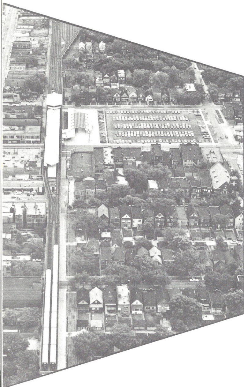
AERIAL VIEW looking east shows Englewood Extension facilities: (from foreground to background) tail track extending to Hermitage, Ashland station platform, transportation office building, bus terminal, parking lot, and expanded car storage yard.
