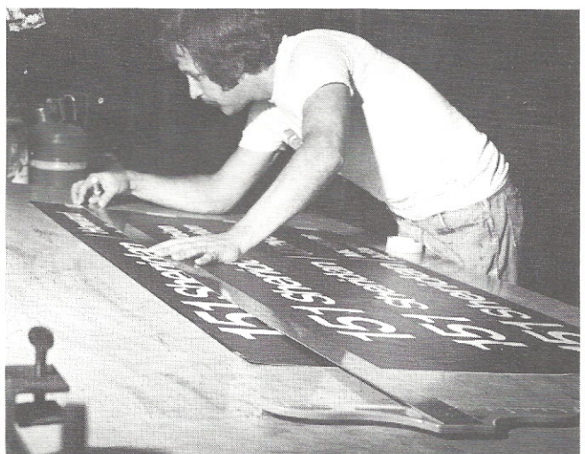
Jeffery Jankus, sign shop painter A, lays out a roller destination sign for use on the No. 151 bus route. (CTA Photos by Eric Blakely)
