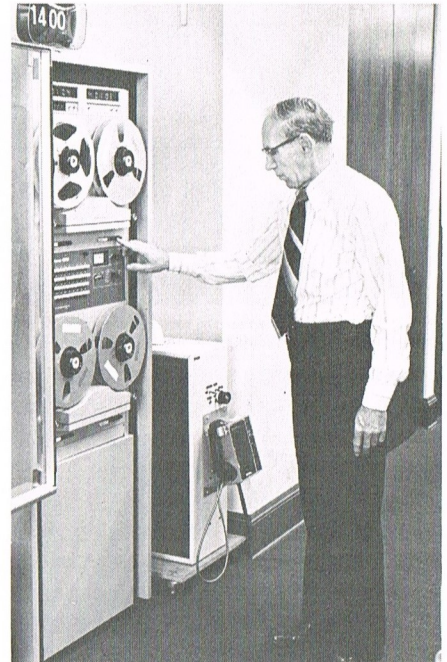
John Leahy checks the tape console that records all voice transmissions between controllers and bus and rail operating personnel and supervisors.
