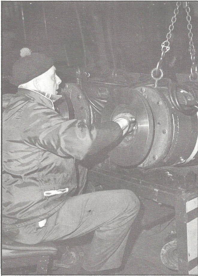
Wally Onysio installs brake disc on rebuilt motor.
