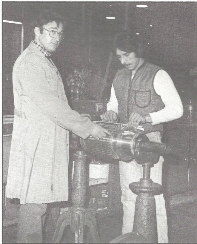
Mark Dondovich, Foreman, and Greg Babicz, Repairman, install new field coils in armature.
