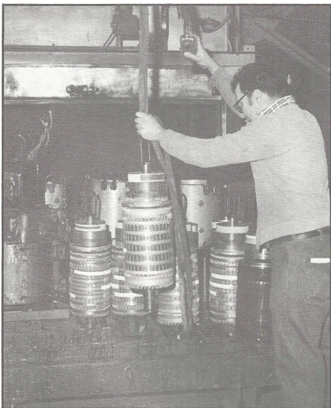
Ralph Gimio prepares motor cases, armatures, and field coils for drying in oven after vacuum pressure impregnation process.
