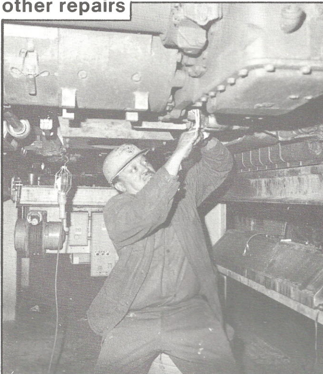
At Howard Shop, Irving Patterson repairs braking system.
