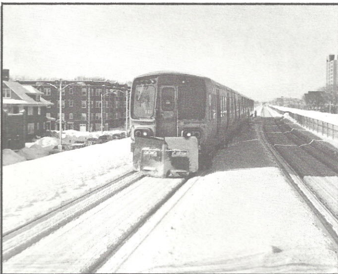
Eastbound train with new snow plow on Lake route near Austin station, Jan. 25. This outer end of the Lake route, on right-of-way of the Chicago and North Western Railway, was one of the embankment areas of CTA operations that had been blocked by snow drifts.
