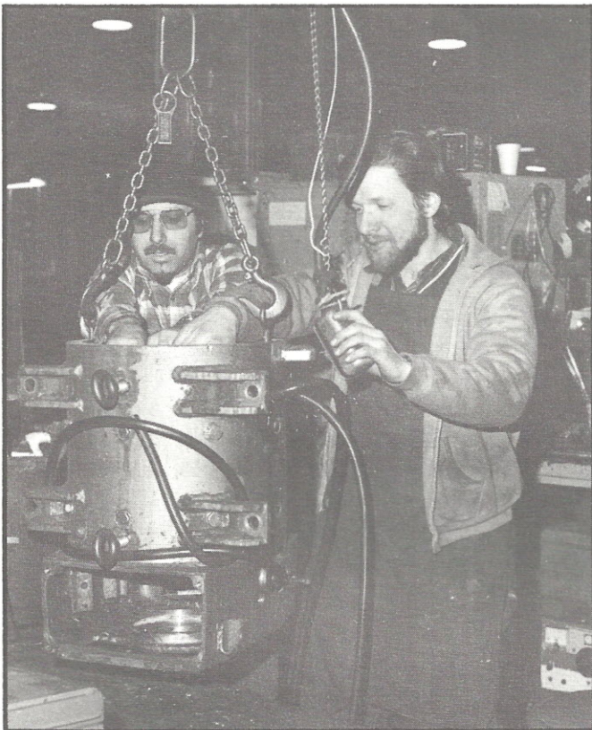
Angelo de Angelis and James Logo prepare motorcase with new field coil for vacuum pressure impregnation process.
