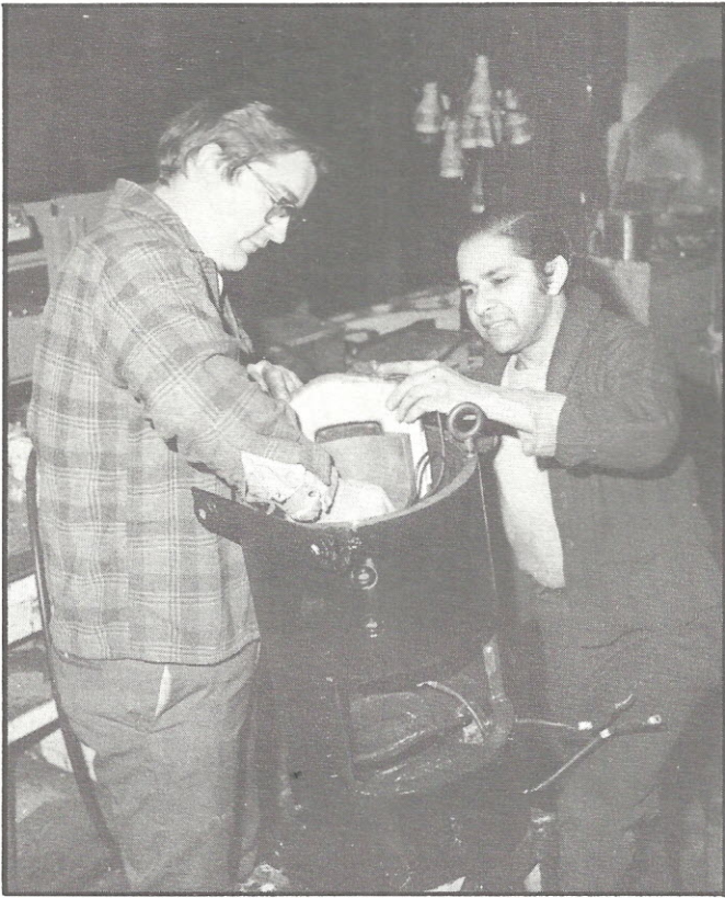
At Skokie Shop, Anthony Torrey and Ranch Patel install field coil in motor generator case.
