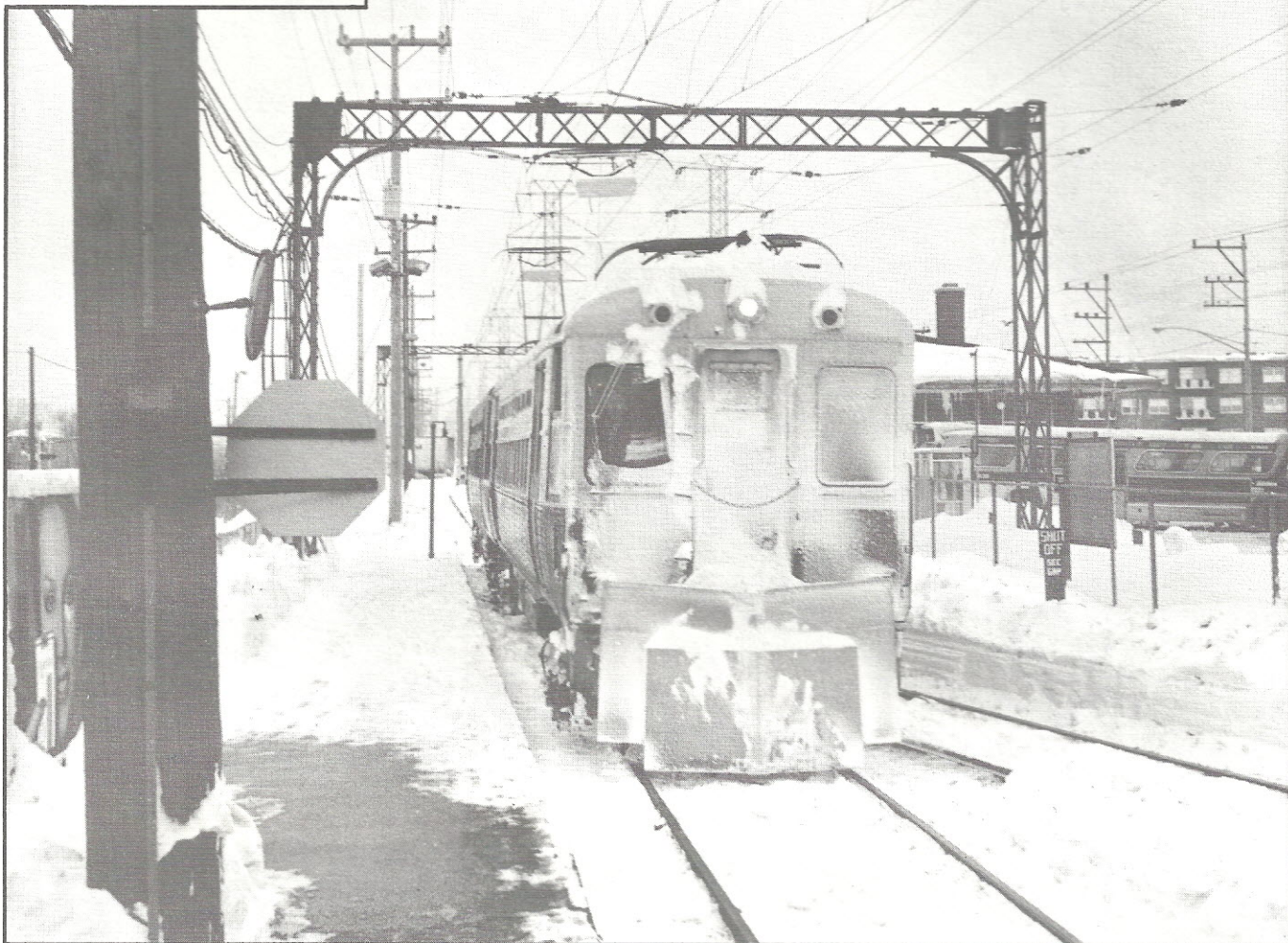
Large snow plows of five layers of heavy plywood were constructed by CTA for high snow drifts that never before had been encountered.
