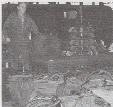
Michael Murphy removing brake drum assembly from motor
