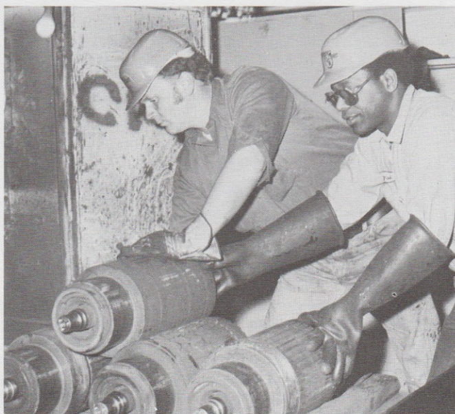
Chester Seymour and Paul Pryor stacking armatures for initial cleaning
