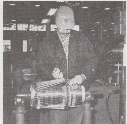
Gary Wilson rewinding armature
