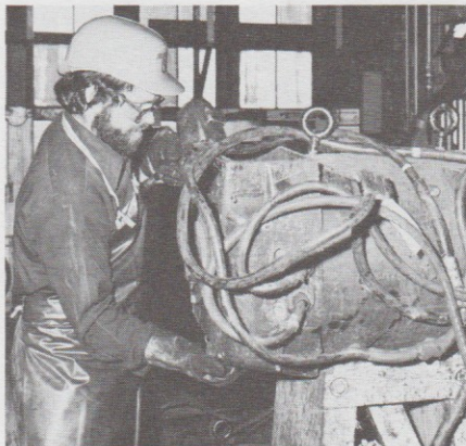
Ray Hagerty removing brush holders in disassembly
