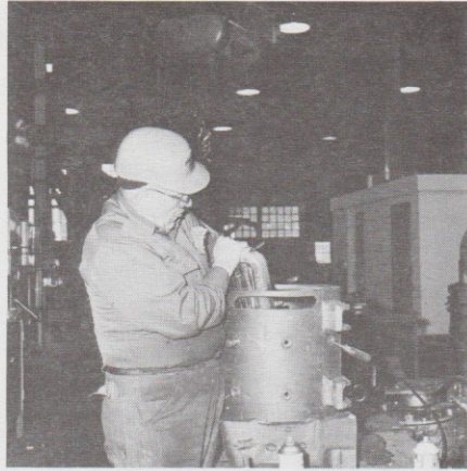
Ray Gunderson installing new field coil
