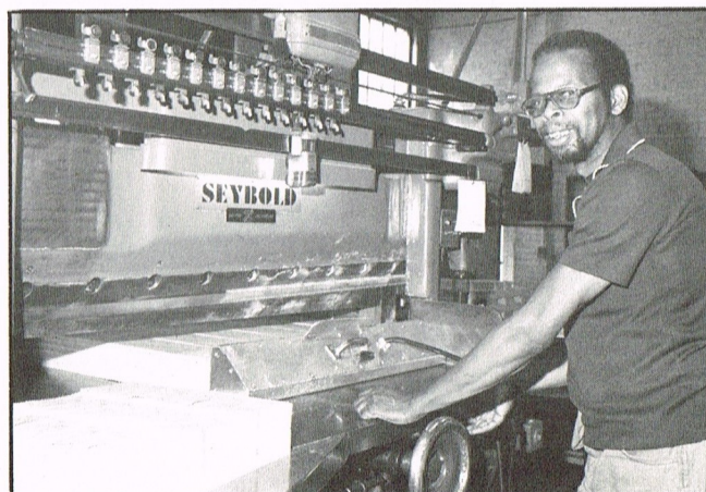
Toby Warmack, paper cutter, slices stitched and joined books into transfer size--5-3/8 inches long, 2-1/4 inches wide.
