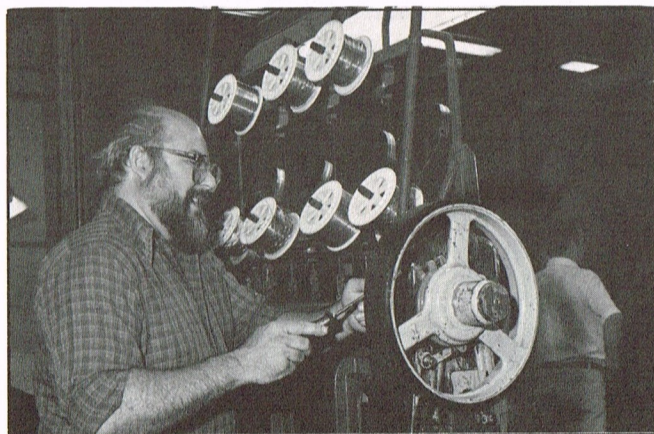
Ron Jareckas, machine shop tool maker, repairs stitching machine. Jareckas and Tony Polich, also a tool maker, keep all print shop machines in running order.
