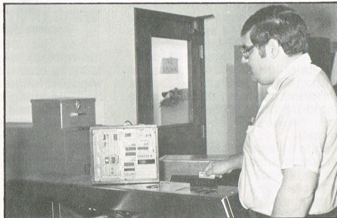
Joe Simonetti demonstrates how an encoded riding card could be slid through "reader" for admittance through turnstile. Component atop turnstile is one of several computer boards used in design of turnstile.
