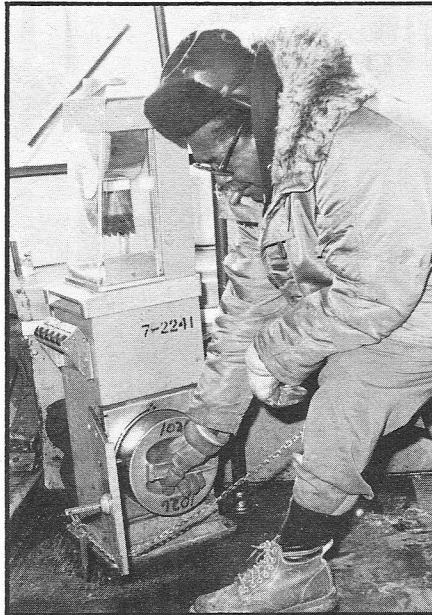
1 Box Puller Marion Henderson demonstrates the process of removing the sealed round cash box from a bus fare box (left). When the cash box is inserted into the self-locking vault opening (right), the money drops into the money vault.
