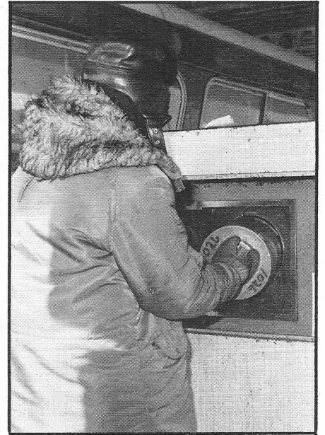
1 Box Puller Marion Henderson demonstrates the process of removing the sealed round cash box from a bus fare box (left). When the cash box is inserted into the self-locking vault opening (right), the money drops into the money vault.
