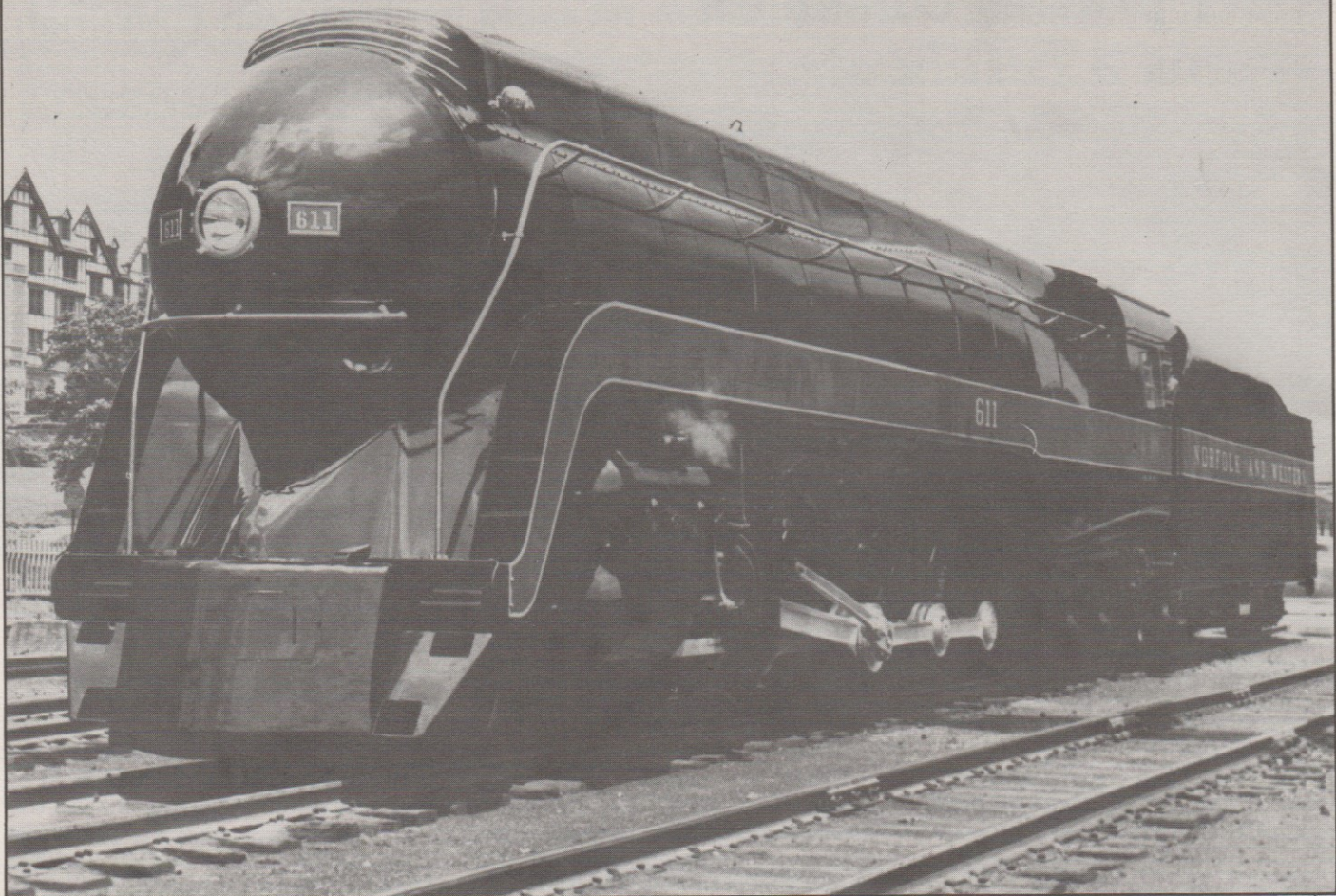
Engine J-611 is out of retirement and back in action. Norfolk and Western's J-Class steam engine, #611, built in 1950 in NW's Roanoke shops, was one of 14 special steam passenger engines used to pull passenger trains in the final days of steam. It produces 5,200 horsepower, twice that of the usual diesel passenger engine. After spending over 20 years in the Roanoke Transportation Museum, the engine was towed to Birmingham, Ala., for a complete overhaul. (Norfolk and Western Railway Photo, courtesy of TRAINS Magazine)
