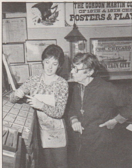
Printers Row Museum volunteer Pam Brown shows Dorothy Martin samples of the metal letters kept in a California type case for use in printing orders on hand-set presses, following a practice that dates back to Gutenberg.
