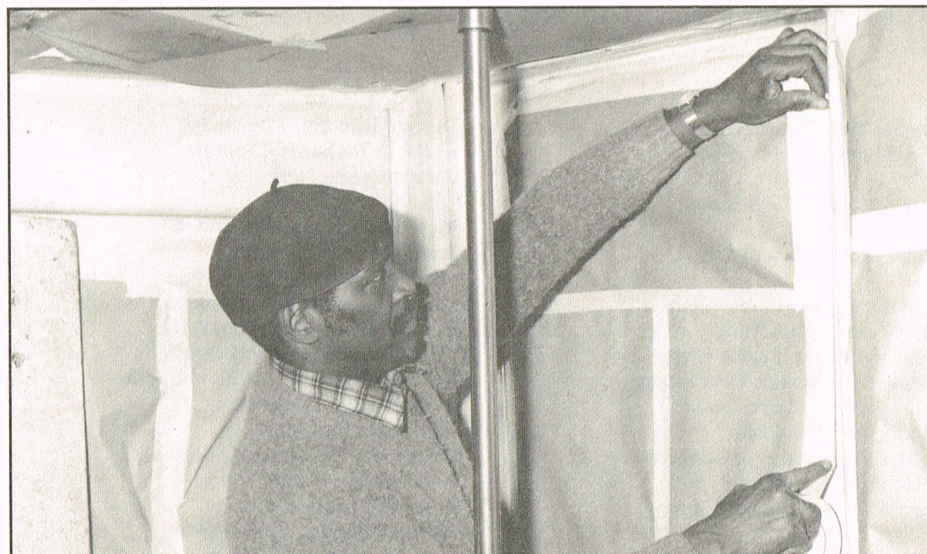
Painter Booker Thomas , completes masking of conductor's window for painting and waxing.
