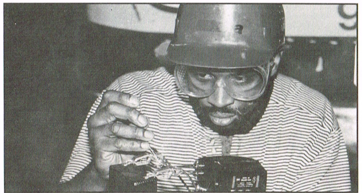
CTA Maintenance Training Center students (left) at Hawthorne are learning proper soldering techniques on bus electrical wiring harnesses. The three-week comprehensive electrical training program instructs bus repairers and line instructors how to troubleshoot and repair electrical defects found on all series of coaches in the CTA bus fleet. Bus repairer Anthony Stewart (right), of Archer garage, demonstrates the sensitive touch and concentration demanded while soldering electrical components.
