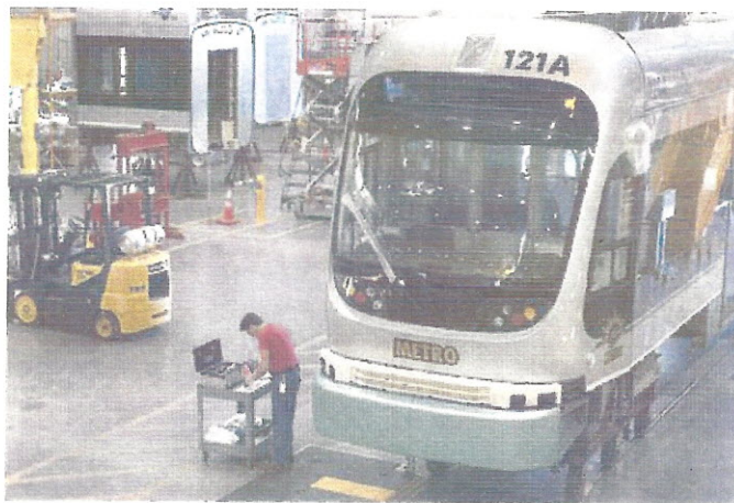
Technician Jeff Song-Collins installs a bumper on a light-rail vehicle Friday at the Metro Operations Facility. The first phase of the light-rail system is scheduled to open to riders in December 2008.
