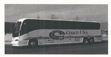
Coach USA has been actively purchasing MCI models for the past three years, upgrading its fleet with the latest innovations. Coach USA ordered its coaches with Cummins engines, ZF Astronic transmissions, Ricon wheelchair lifts and Amaya seats with three-point seatbelts. The new coaches will also feature Amerex fire suppression systems and provisions for GPS installation.
