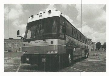
CEC's new MCI ISTVs seat 61 inmates with multiple segregation areas and come with GPS tracking and a surveillance system. The coaches, which are built on the MCI D4000 platform, additionally feature Detroit Diesel engines and Allison transmissions. The vehicles are in use at Johnson County Jail, Cleburne, Texas, a CECmanaged facility.
