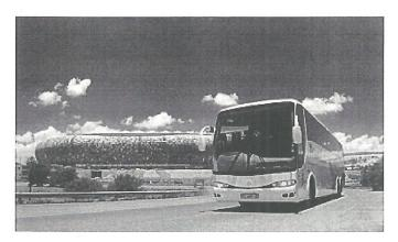
The Mercedes-Benz O 500 RSD is equipped with a fully electronic management engine with 260 kW output of power. The vehicles will be fitted with a fully automatic transmission with integrated retarder, which has recently been introduced to the product range. The automatic transmission has a number of driving and safety benefits, as it allows the driver to concentrate on stress-free-driving, with the gearbox shifting automatically on demand, and is ideal for inter-city transportation.
