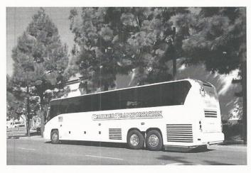
Certified's new J4500 coach, featuring a 2010 EPA Cummins ISX 11.9L 425 hp engine paired with an Allison B500 transmission, also helps the company comply with the state's emission regulation. Cummins estimates the engine also offers up to five percent improved fuel efficiency compared to 2007 engines, depending on duty cycle. It's quieter, too.
