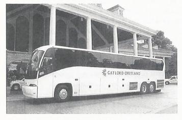
The new coaches have Detroit Series 60 engines and Allison B500 transmissions; seating with three-point safety belts; Braun wheelchair lifts; and an ASA color back-up camera. The Blaupunkt Enhanced Audio System and six 15.4-inch LCD widescreen monitors allow the company to show promotional and
