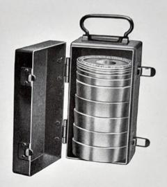
The Ashton Tester body is of bronze, nickel plated and, with fittings, is neatly packed in a welded steel box, with lock, having serviceable dull black finish. The weights also are in a similar box (or boxes) each of which has handle for convenience in carrying.
