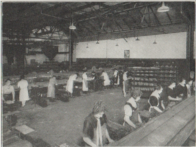
Core Room containing 60 benches and 6 gas-fired ovens. An asbestos screen deflects the oven heat away from the workers.
