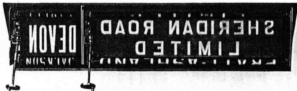
Rear View Special Type Destination and Route Sign for Double Deck Buses. No. S-551 LLB
