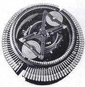
closed gear unit operating in bath of oil. Resistance mounted on periphery of barrel.
