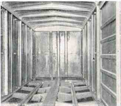
Interior construction of light-weight box car.
