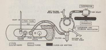
Because Propane enters the engine as a gas and not as a liquid, there is no dilution of crankcase oil. Oil change periods are extended to about twice that of a gasoline or diesel engine. There is less ring, piston and cylinder wear, which prolongs the intervals between motor overhauls. Propane burns clean and completely, leaving no carbon deposits, no smoke, no obnoxious exhaust odors. The cost of Propane is less than the cost of gasoline,
