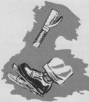
WHEN THE HAND BRAKE IS SET, THE ACCELERATOR PEDAL IS DIFFICULT TO DEPRESS
