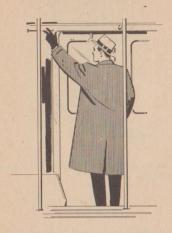
1 Signal operator for your stop; stand on treadle step. Your weight on treadle step will activate the door when operator positions door-opening switch.
