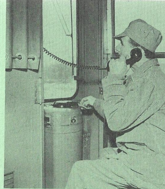
CTA motorman uses train-phone communications system aboard North-South "L"-subway train. Since the motorman can speak directly with central control and dispatching personnel in the Merchandise Mart offices, he is able to report at once any instances, such as illness of a passenger, equipment failure, disturbance or other situations which cause delays and gaps in service.
