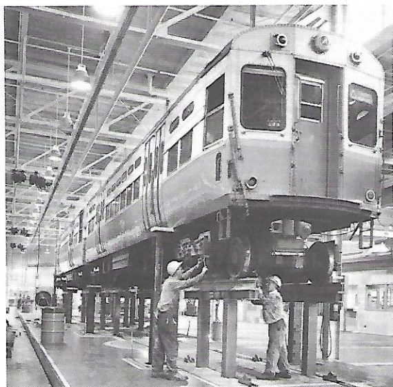
Hoists in the Congress Terminal inspection shop can lift a two-car train five feet off tracks for maintenance or removal of trucks.
