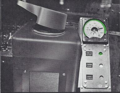
Speedometer segments light up to show allowable speed ranges.
