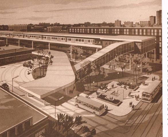
Convenient undercover interchange between buses and rapid transit will result from modernization of the Jackson Park terminal of the North-South route at 63rd/Stony Island. The present facility, basically unchanged since 1893, will be replaced by a modern station with escalators to street level, radiant platform heating and fluorescent lighting. The bus turnaround will eliminate operation over neighborhood side streets.
